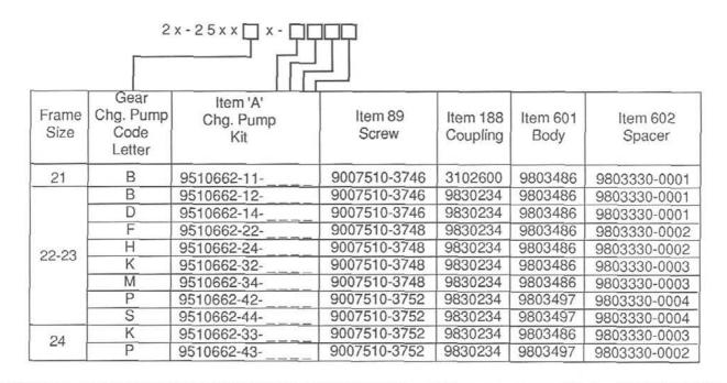
CAUTION: If the unit has an Electrical Displacement Control (EDC), the charge pump kit ordered MUST be one without an orifice.
